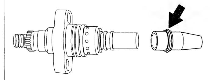
Slip support ring/O-ring/support ring with outer part of assembly device 0 986 612 495 onto assembly (picture).
